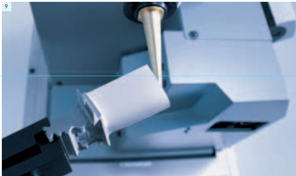
LASERTEC 80 Shape: |7| Insertion of the bevelled exit holes with mill-lasering |8| Shape machine version with 2 laser sources (1 boring and 1 milling laser) |9| Technology combination: laser boring of the cylindrical duct (step 1), incorporation of the bevelled exit holes with the milling laser (step 2)
